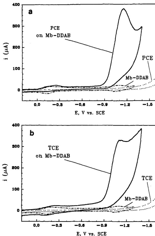
**Figure 4.** Steady state cyclic voltammograms at 100 mV s<sup>-1</sup> in pH 5.5 buffer + 50 mM NaBr: (a) Mb-DDAB films on PG with and without 12 mM PCE, and PCE on a DDAB-PG electrode without Mb; (b) Mb-DDAB films on PG with and without 30 mM TCE, and TCE on a DDAB-PG electrode without Mb.
