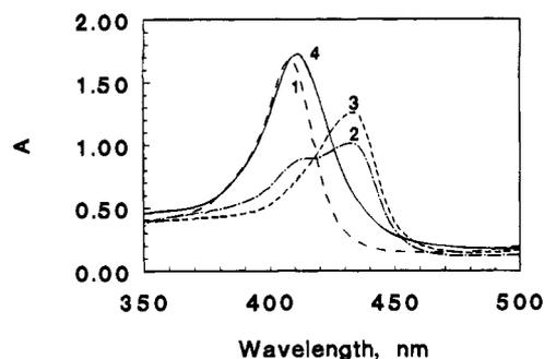
**Figure 2.** Spectroelectrochemistry of Mb-DDAB films on a tin-doped indium oxide electrode in a pH 5.5 buffer + 50 mM NaBr containing no Mb. Spectra were taken after the following potentials vs SCE were applied for 20 min: (1) 100, (2)  $-250$ , (3)  $-500$ , and (4)  $-1250 \text{ mV}$ . Film thickness 15–20  $\mu\text{m}$ .
