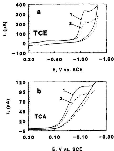
**Figure 7.** First CV scan after equilibration (1) and steady state scan after repetitive cycling (2) of Mb-DDAB electrodes in pH 5.5 buffer + 50 mM NaBr containing (a) 30 mM trichloroethylene and (b) 10 mM trichloroacetic acid.
