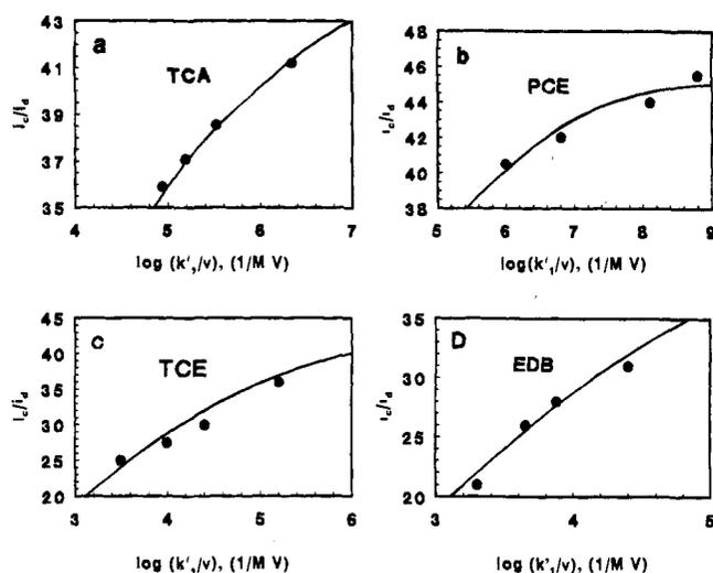
**Figure 8.** Catalytic efficiencies as  $i_c/i_d$  vs  $\log(k_1'/\nu)$  for Mb-DDAB films in 10 mM organohalide solutions plotted (●) for average  $k_1'$  values (Table 6) for (a) trichloroacetic acid, (b) tetrachloroethylene, (c) trichloroethylene, and (d) ethylene dibromide. Lines represent theoretical predictions simulated in relevant ranges of  $k_1'/\nu$  by using the EC' mechanism with SET approximation (see Experimental Section).
