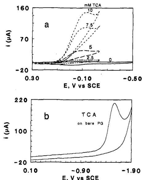
**Figure 3.** Steady state cyclic voltammograms at 100 mV s<sup>-1</sup> in pH 5.5 buffer + 50 mM NaBr: (a) Mb-DDAB films with trichloroacetic acid at 0, 2.5, 5, 7.5, and 10 mM; (b) reduction peak for 10 mM TCA on a DDAB-PG electrode (no Mb).
