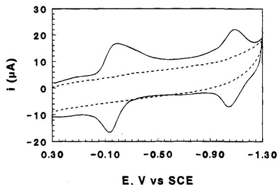
**Figure 1.** Steady state cyclic voltammograms at  $100 \text{ mV s}^{-1}$  in pH 5.5 buffer + 50 mM NaBr: dashed line, bare PG electrode with 0.5 mM Mb in solution; solid line, fully loaded Mb-DDAB film in buffer containing no Mb.
