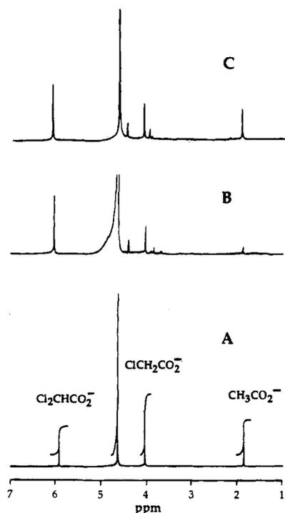
**Figure 6.** NMR spectra of products from Mb-DDAB-catalyzed reduction of 25 mM TCA in 10 mM deuterated acetate buffer + 50 mM NaBr at pH 5.5 at  $-0.4$  V vs SCE: (a) standards dichloroacetate, monochloroacetate, and acetate, (b) after electrolysis for 5 h, and (c) after electrolysis for 24 h.
