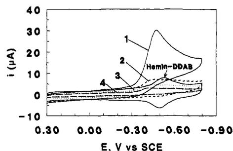
**Figure 5.** Cyclic voltammograms at 100 mV s<sup>-1</sup> in pH 5.5 buffer + 50 mM NaBr for hemin-DDAB films with and without 10 mM trichloroacetic acid, showing the instability of reduction current after the first scan. (1) first scan, (2) second scan, (3) third scan, (4) fourth scan. CV without trichloroacetic acid present is labeled hemin-DDAB.
